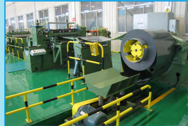
CRGO slitting line
